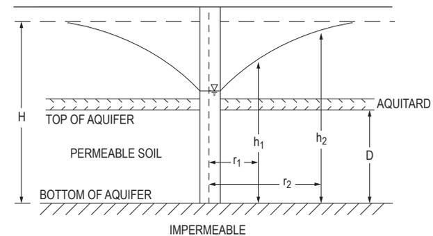
$$Q = \frac{2\pi T (h_2 - h_1)}{\ln\left(\frac{r_2}{r_1}\right)}$$
