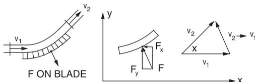
$$-F_x = Q\rho(v_2 \cos \alpha - v_1)$$
