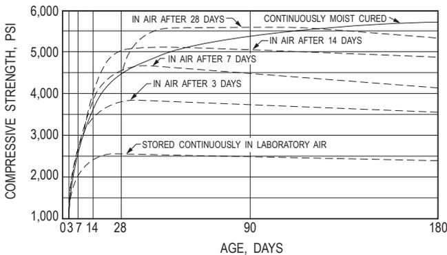
Concrete compressive strength varies with moist-curing conditions. Mixes tested had a water-cement ratio of 0.50, a slump of 3.5 in., cement content of 556 lb/yd<sup>3</sup>, sand content of 36%, and air content of 4%.
