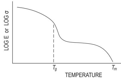
The above curve shows the temperature dependent strength ( $\sigma$ ) or modulus ( $E$ ) for a thermoplastic polymer.
