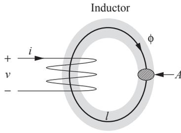
The inductance  $L$  (henrys) of a coil of  $N$  turns wound on a core with cross-sectional area  $A$  ( $\text{m}^2$ ), permeability  $\mu$  and flux  $\phi$  with a mean path of  $l$  (m) is given as:
