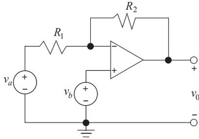
$$v_0 = -\frac{R_2}{R_1} v_a + \left(1 + \frac{R_2}{R_1}\right) v_b$$
