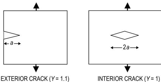
The critical value of stress intensity at which catastrophic crack propagation occurs,  $K_{IC}$ , is a material property.
