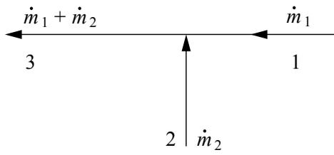
$$\dot{m}_1 h_1 + \dot{m}_2 h_2 = h_3 (\dot{m}_1 + \dot{m}_2)$$
