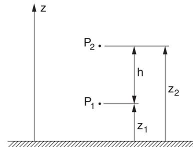
The difference in pressure between two different points is
