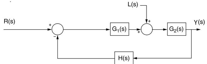
where  $G_1(s)$  is a controller or compensator,  $G_2(s)$  represents a plant model, and  $H(s)$  represents the measurement dynamics.  $Y(s)$  represents the controlled variable,  $R(s)$  represents the reference input, and  $L(s)$  represents a disturbance.  $Y(s)$  is related to  $R(s)$  and  $L(s)$  by
