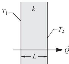
$$\dot{Q} = \frac{-kA(T_2 - T_1)}{L}, \text{ where}$$
