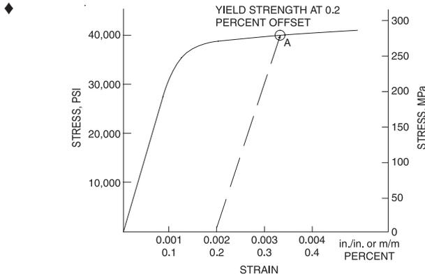
The slope of the linear portion of the curve equals the modulus of elasticity.
