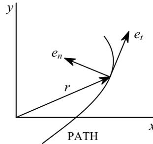
Unit vectors  $\mathbf{e}_t$  and  $\mathbf{e}_n$  are, respectively, tangent and normal to the path with  $\mathbf{e}_n$  pointing to the center of curvature. Thus
