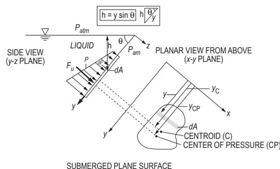
The pressure on a point at a vertical distance  $h$  below the surface is:
