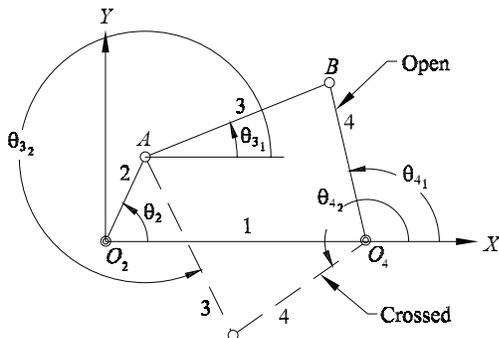
The four-bar linkage shown above consists of a reference (usually grounded) link (1), a crank (input) link (2), a coupler link (3), and an output link (4). Links 2 and 4 rotate about the fixed pivots  $O_2$  and  $O_4$ , respectively. Link 3 is joined to link 2 at the moving pivot  $A$  and to link 4 at the moving pivot  $B$ . The lengths of links 2, 3, 4, and 1 are  $a$ ,  $b$ ,  $c$ , and  $d$ , respectively.
