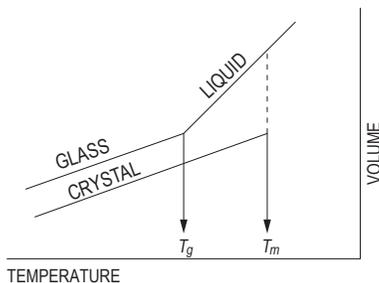
The volume-temperature curve as shown above is often used to show the difference between amorphous and crystalline solids.
