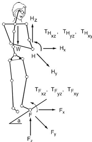
The coefficient of friction  $\mu$  and the angle  $\alpha$  at which the floor is inclined determine the equations at the foot.
