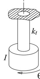
For torsional free vibrations it may be shown that the differential equation of motion is
