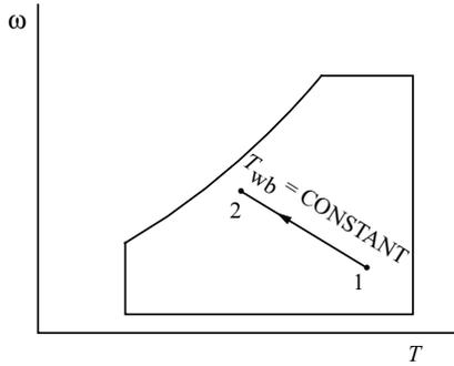
$$h_2 = h_1 + h_3(\omega_2 - \omega_1)$$
