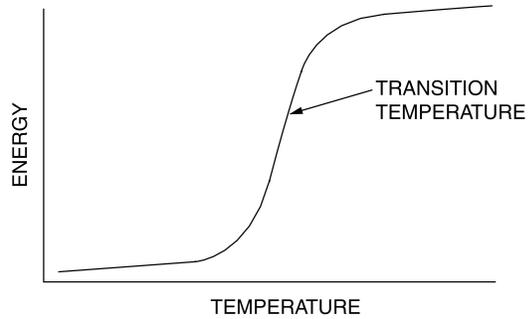
Impact tests determine the amount of energy required to cause failure in standardized test samples. The tests are repeated over a range of temperatures to determine the *ductile to brittle transition temperature*.
