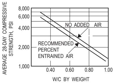
Concrete strength decreases with increases in water-cement ratio for concrete with and without entrained air.
