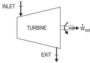
For an adiabatic turbine with  $\Delta PE = 0$  and negligible  $\Delta KE$ :
