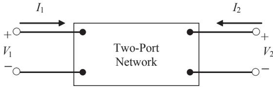
A two-port network may be represented by an equivalent circuit using a set of two-port parameters. Three commonly used sets of parameters are impedance, admittance, and hybrid parameters. The following table describes the equations used for each of these sets of parameters.
