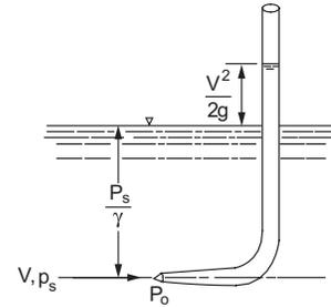
For a *compressible fluid*, use the above incompressible fluid equation if the Mach number  $\leq 0.3$ .
