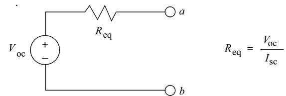
The open circuit voltage  $V_{\text{oc}}$  is  $V_a - V_b$ , and the short circuit current is  $I_{\text{sc}}$  from  $a$  to  $b$ .
