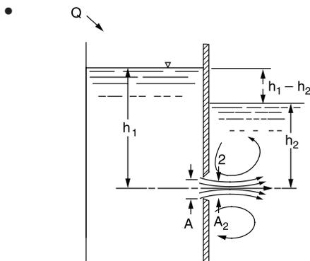
$$Q = A_2 v_2 = C_c C_v A \sqrt{2g(h_1 - h_2)}$$
