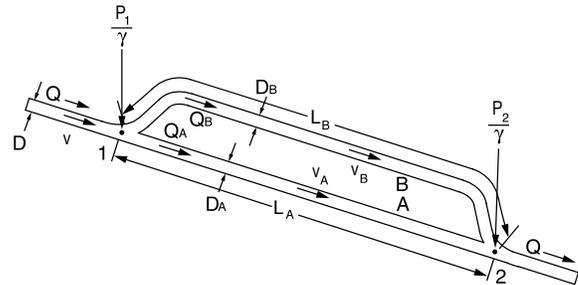
For pipes in parallel, the head loss is the same in each pipe.
