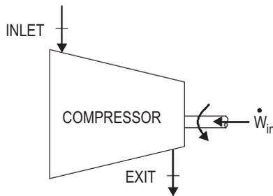
For an adiabatic compressor with  $\Delta PE = 0$  and negligible  $\Delta KE$ :
