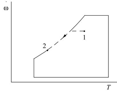
$$\dot{Q}_{out} = \dot{m}_a[(h_1 - h_2) - h_{f3}(\omega_1 - \omega_2)]$$
