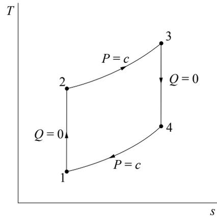
$$w_{12} = h_1 - h_2 = c_p (T_1 - T_2)$$
