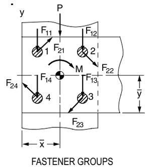
The location of the centroid of a fastener group with respect to any convenient coordinate frame is:
