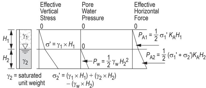
Active forces on retaining wall per unit wall length (as shown):
