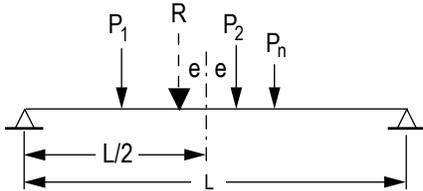
The **absolute maximum moment** produced in a beam by a set of "n" moving loads occurs when the resultant "R" of the load set and an adjacent load are equal distance from the centerline of the beam. In general, two possible load set positions must be considered, one for each adjacent load.
