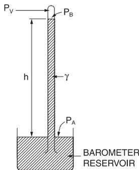
$P_v$  = vapor pressure of the barometer fluid
