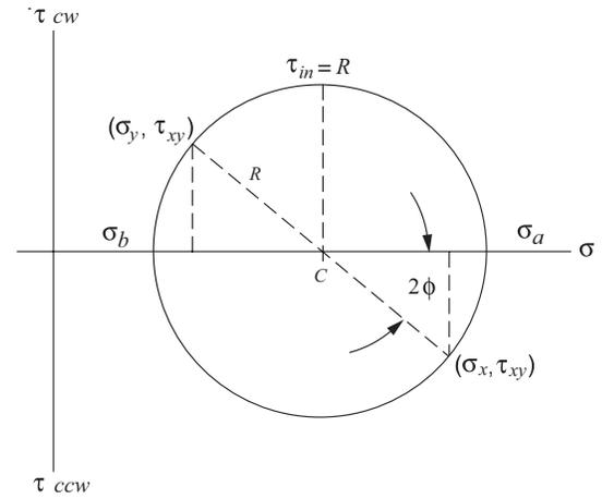
The maximum *inplane* shear stress is  $\tau_{in} = R$ . However, the maximum shear stress considering three dimensions is always
