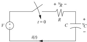
$$t \geq 0; v_C(t) = v_C(0)e^{-t/RC} + V(1 - e^{-t/RC})$$
