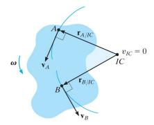
3. Given the magnitude and direction of two parallel velocities  $\vec{v}_A$  and  $\vec{v}_B$ . Here the location of the IC is determined by proportional triangles. Examples are shown in the figure below. In both cases  $r_{A/IC} = v_A/w$  and  $r_{B/IC} = v_B/w$ . If d is a known distance between points A and B then in the example to the left  $d = r_{A/IC} + r_{B/IC}$  and in the example to the right  $d = r_{B/IC} - r_{A/IC}$
