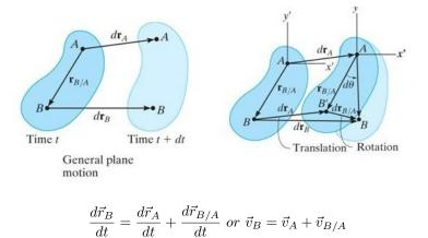
The magnitude of  $\vec{v}_{B/A}$  is  $r_{B/A} d\theta/dt$  and its direction is along the z' axis.
