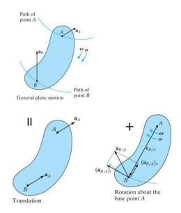
Since the relative acceleration components represent the effect of circular motion observed from translating axes having their origin at the base point A, these terms can be expressed as  $(\vec{a}_{B/A})_t = \vec{\alpha} \times \vec{r}_{B/A}$ and  $(\vec{a}_{B/A})_n = -\omega^2 \vec{r}_{B/A}$
