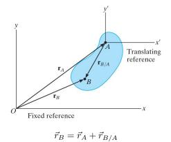
During time dt, points A and B undergo displacements  $d\vec{r}_A$  and  $d\vec{r}_B$  such that
