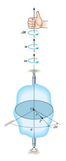
• Angular velocity: Measures the time rate of change of the angular position. If  $\theta$  is the angular position of a radial line located in some representative plane of the body, the angular velocity  $\omega$  is along the axis of rotation and its direction can be determined using the right hand rule; that is, the fingers of the right hand are curled with the sense of rotation, the thumb indicate the direction of the angular velocity.
