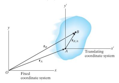
A and B are two points in the rigid body. Because our object is a rigid body, all its points are at fixed distances from each other, moreover, for planar rigid body translation the direction  $\vec{r}_{A/B}$  is constant then  $(d\vec{r}_{B/A}/dt = 0 \text{ and } d^2\vec{r}_{B/A}/dt^2 = 0)$ . We have the following relations:
