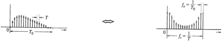
$$f_0 = \frac{1}{T_0} \quad N = \frac{T_0}{T} \quad N = \frac{f_s}{f_0} \quad f_0 = \frac{f_s}{N}$$
