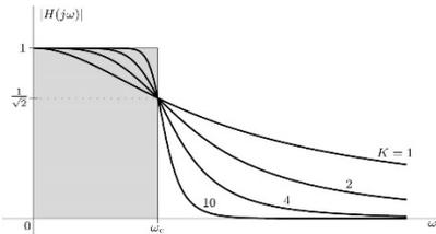
$$|H(j\omega)| = \frac{1}{\sqrt{1 + \left( \frac{\omega}{\omega_c} \right)^{2K}}} \quad H(s) = \frac{\omega_c^K}{\prod_{k=1}^K (s - p_k)}$$
