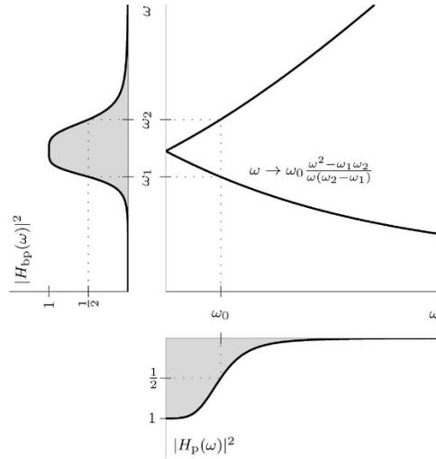
$$s \rightarrow \omega_0 \frac{s^2 + \omega_1 \omega_2}{s(\omega_2 - \omega_1)} \quad \text{OR} \quad \omega \rightarrow \omega_0 \frac{\omega^2 - \omega_1 \omega_2}{\omega(\omega_2 - \omega_1)}$$
