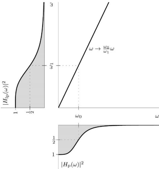
$$s \rightarrow \frac{\omega_0}{\omega_1} s \quad \text{OR} \quad \omega \rightarrow \frac{\omega_0}{\omega_1} \omega$$
