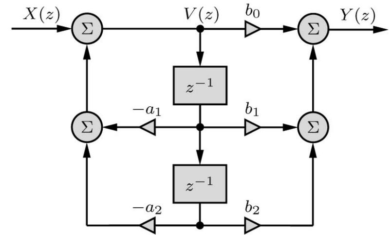
DFII is **canonic** since the number of delays equal to the order of the transfer function.
