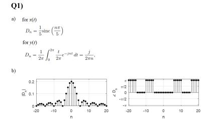
c) For x(t), the 5<sup>th</sup> hormonic will be less than 10% of the DC and the approximate power for the DC and the first five harmonics is P = 0.1805. For y(t), the 2<sup>nd</sup> hormonic will be less than 10% of the DC and the approximate power for the DC and the first two harmonics is P = 0.3013.
